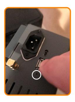
3. While holding the button depressed, connect the AC line chord to power up the charger.
