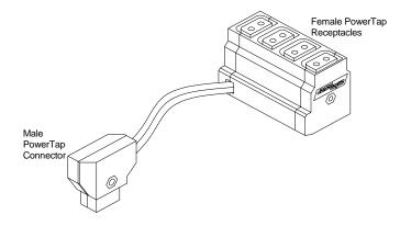
Note: Check your Gold Mount battery adapter for maximum current draw. <u>All</u> Anton/Bauer<sup>®</sup> Gold Mounts will have a maximum current draw of between 7 and 10 amps.
